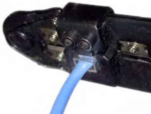
Fig 1.12 Crimping of wire
